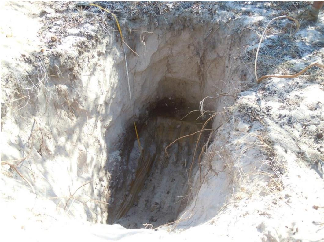
**Figure 17.** KO8. Pale sand on dark band with ferruginous nodules on weathered Malmesbury Group bed rock. 1 Silcrete core @  $\pm 1.2\text{m}$  in sand and ferruginous nodules. The shine may be polish, which suggests that it may have been exposed to the wind previously or under water.
