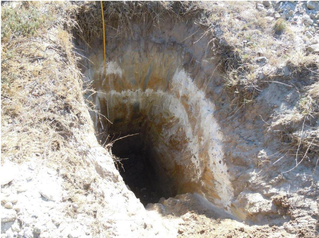
**Figure 19.** KO9. Pale grey sand over ferruginous nodules and apparently-mixed calcrete lenses and weathered Malmesbury Group rock on weathered Malmesbury Group bed rock.
