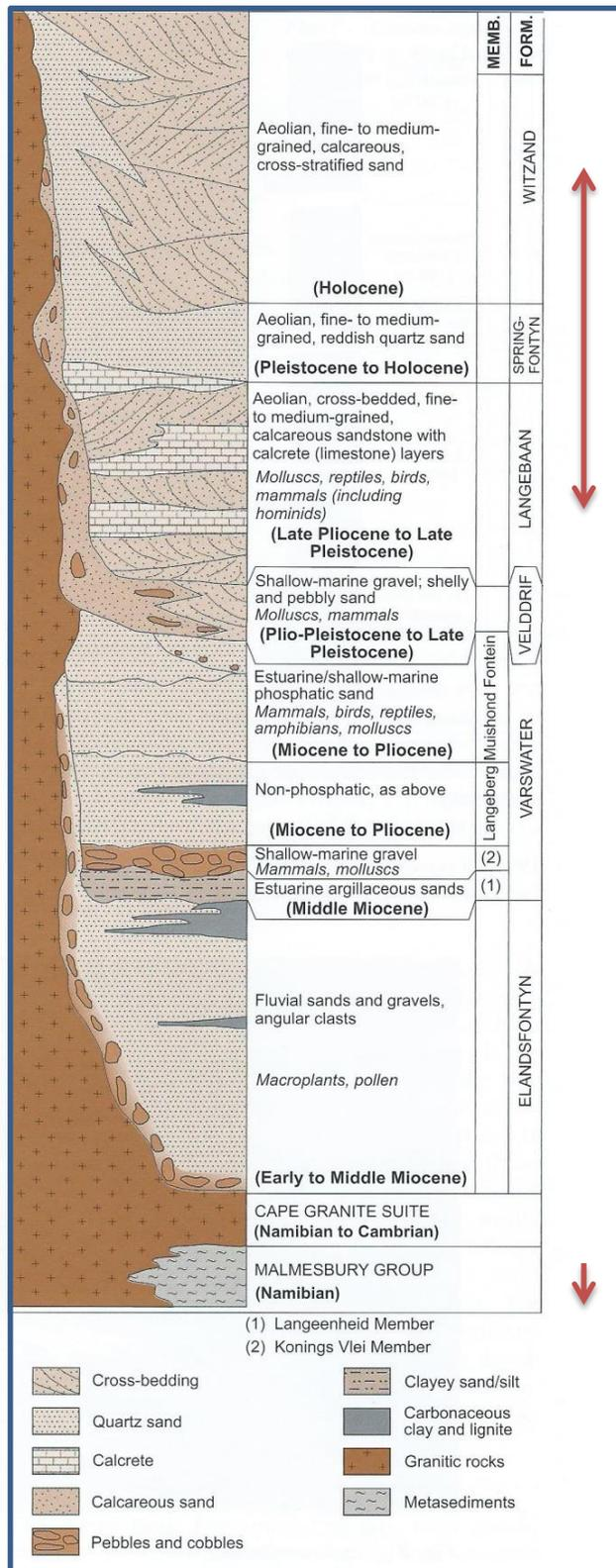
**Figure 4.** Generalized section through the Sandveld Group (Roberts, et al., 2006), figure 10: 616. Arrows indicate formations most likely to be expected in the test pits.
